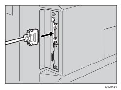
2 Attach the other end of the parallel cable to the port of the computer. Secure the cable.
